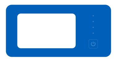
Resin Dome Size: 49.97mm x 29.94mm. Radius Corner: 3mm Magnenta line does not print! This is the cutter guide
