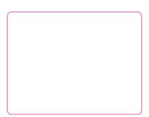
Resin Dome Size: 52mm x 39.5mm. Radius Corner: 2.5mm Magnenta line does not print! This is the cutter guide
